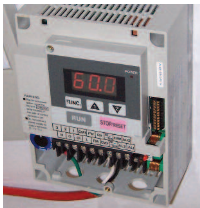
Figure 36: Variable Frequency Drive (VFD).
